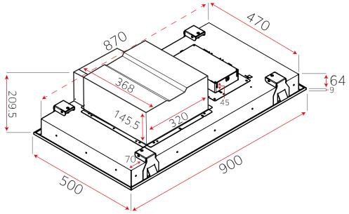
Ducting – Our slimline motor is designed with a rectangular ducting system. Please note as this ducting is rectangular and not round, it will have different dimensions.
